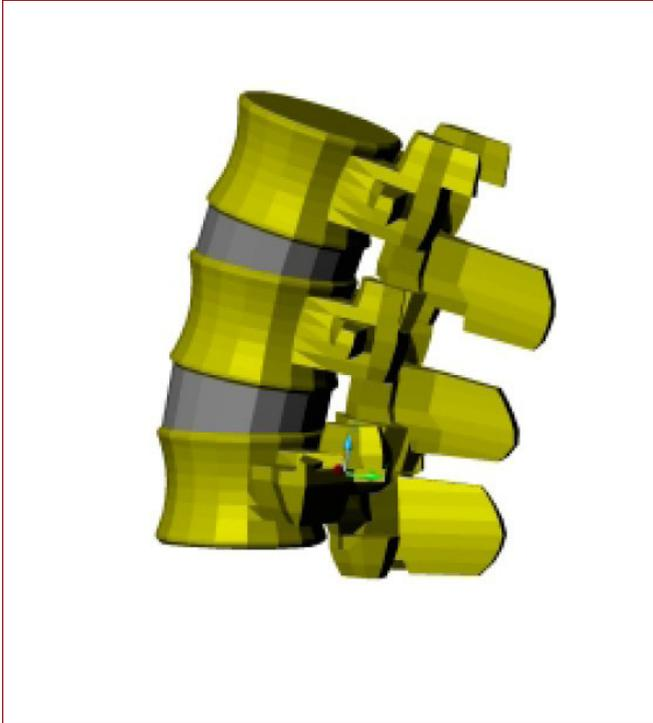
Ligaments were modeled as two-point elements counteracting to pulling, and the locations were arranged according to anatomical data obtained from the literature. Ligament sectional areas were taken from the literature and are described in Table-1.
