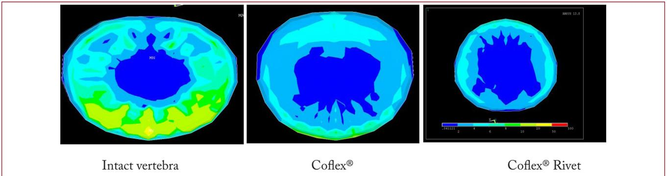
On extension, it was recorded as an average of 5.26 MPa in a normal disc, 3.20 MPa with Coflex® and 3.16 MPa with Coflex® Rivet. According to these data, it was observed that Coflex® reduced the load on the disc at a ratio of 39% and Coflex® Rivet reduced it at a ratio of 40% (Figure-7).
