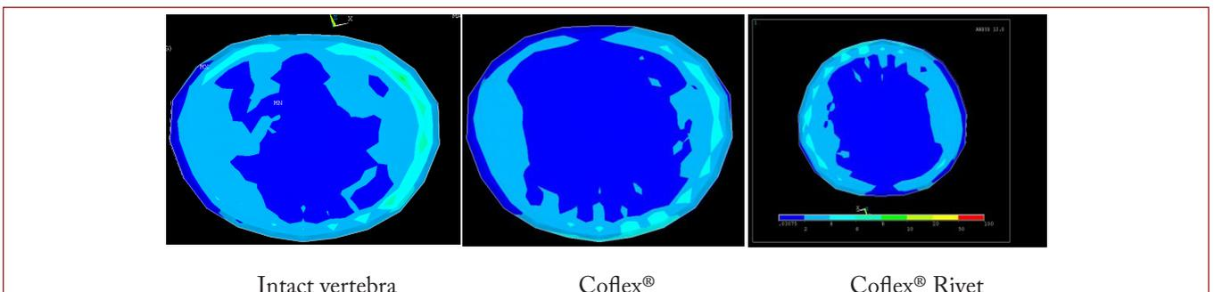
On rotation, the loading was recorded as 4.4 MPa in a normal disc, 5.2 MPa with Coflex® and 5.2 MPa with Coflex® Rivet. In the light of these findings, Coflex® Rivet and Coflex® reduced disc loading at a ratio of 32%.
