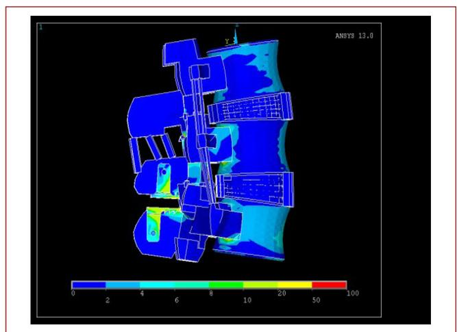
**Figure-4.** Front view of all movements after loading in the Coflex®-applied model
