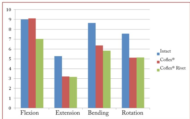
On flexion, it was recorded as an average of 8.98 MPa in a normal disc, 9.11 MPa with Coflex® and 7.03 MPa with Coflex® Rivet. According to these data, it was observed that Coflex® increased the load on the disc at a ratio of 1%, and Coflex® Rivet reduced the load on the disc at a ratio of 22% (Figure-6).
