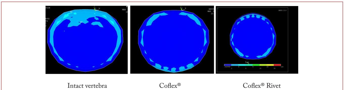
On bending, the loading was recorded as 8.7 MPa in a normal disc, 6.4 MPa with Coflex® and 5.8 MPa with Coflex® Rivet. In the light of these data, it was observed that Coflex® Rivet reduced disc loading at a ratio of 34% and Coflex® reduced it at a ratio of 26% (Figure-8).
