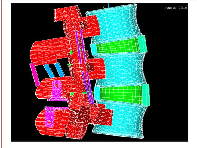
The intact model was composed of 77,283 connection points and 48,173 elements. The Coflex®-applied model was composed of 71,594 connection points and 43,076 elements<sup>1,12</sup>.
