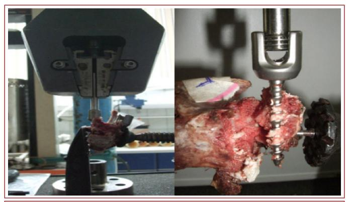
**Figure-3.** Biomechanical test was performed after 12 hours of keeping the vertebraes in room temperature. Screw pullout test was applied to pedicle screws for biomechanical testing.
